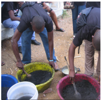
5. Mixing binder, water and charcoal to make briquettes
