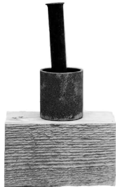
Charcoal Press ($2) – presses carbonized material into charcoal briquettes at speeds of up to 10-15 briquettes per minute. Briquettes pressed by hands crumble.
