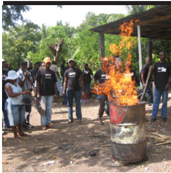
2. Carbonizing agricultural waste by burning it in an oil drum
