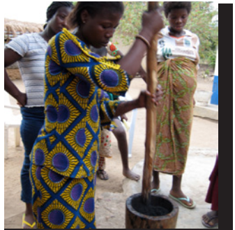
4. Crushing carbonized corn cobs into a powder
