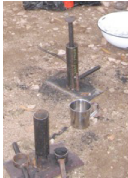
First Prototype $30 4-5 Briquettes a Minute
